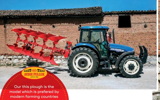
Our this plough is the model which is prefered by modern farming countries due to its time fuel saving feature. In reversible ploughs number of nuts and bolts on mouldboard are less than on other ploughs. So it lasts longer.
